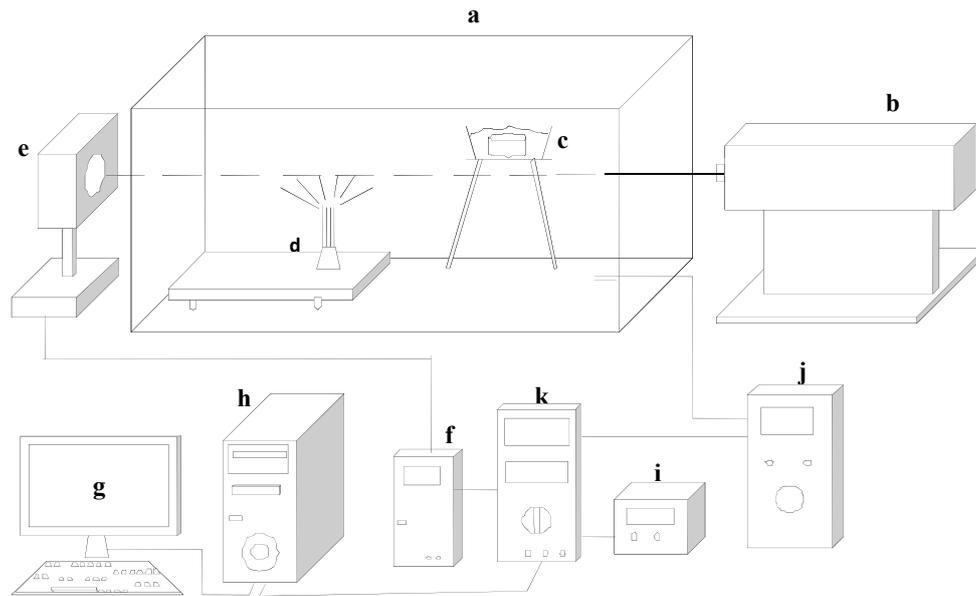
**Fig. 2.** Illustration of experimental system (a) Glass container (b) He-Ne LASER (c) Ultrasonic water fogger (d) NAI generator (e) Receiver (f) Light Intensity meter (g-h) Computer (i) Timer (j) Air ion counter (k) Data logger.
