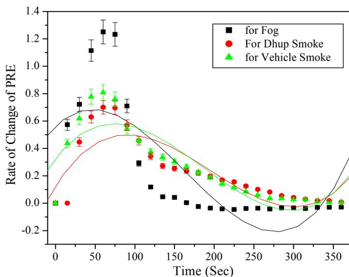
**Fig. 6.** Rate of change of particle removal efficiency verses time for Fog, Dhup Smoke and Vehicle Smoke.
