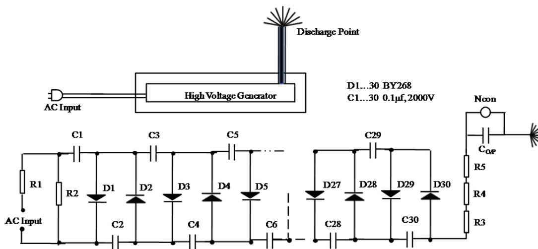
Fig. 1. Schematic of an air ion generator.
