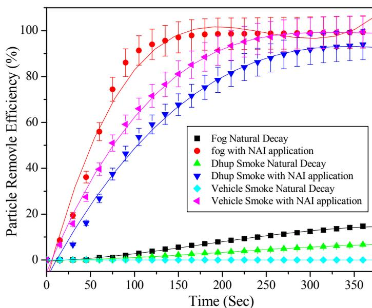
**Fig. 5.** Particle removal efficiency verses time with natural decay and NAI application for Fog, Dhup Smoke and Vehicle Smoke.
