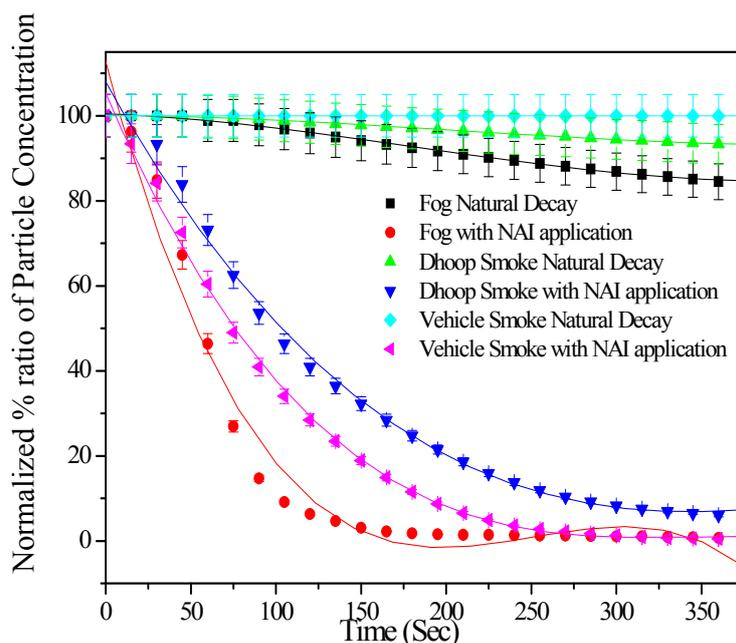
**Fig. 4.** Particle concentration decay (normalized %) versus time with natural decay and NAI application for Fog, Dhoop Smoke and Vehicle Smoke.
