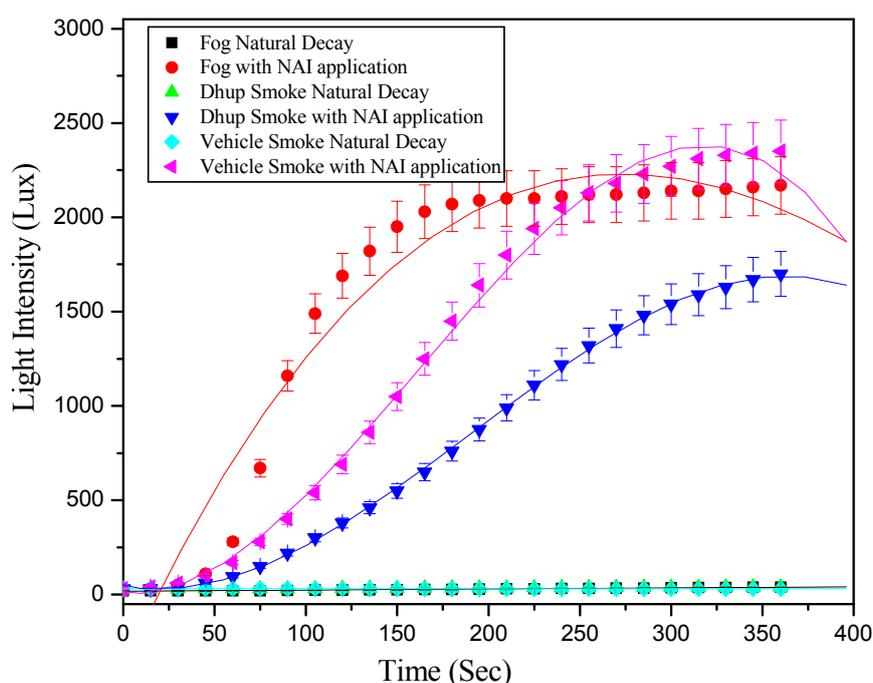
**Fig. 3.** Light intensity variation versus time with natural decay and NAI application for Fog, Dhoop Smoke and Vehicle Smoke.
